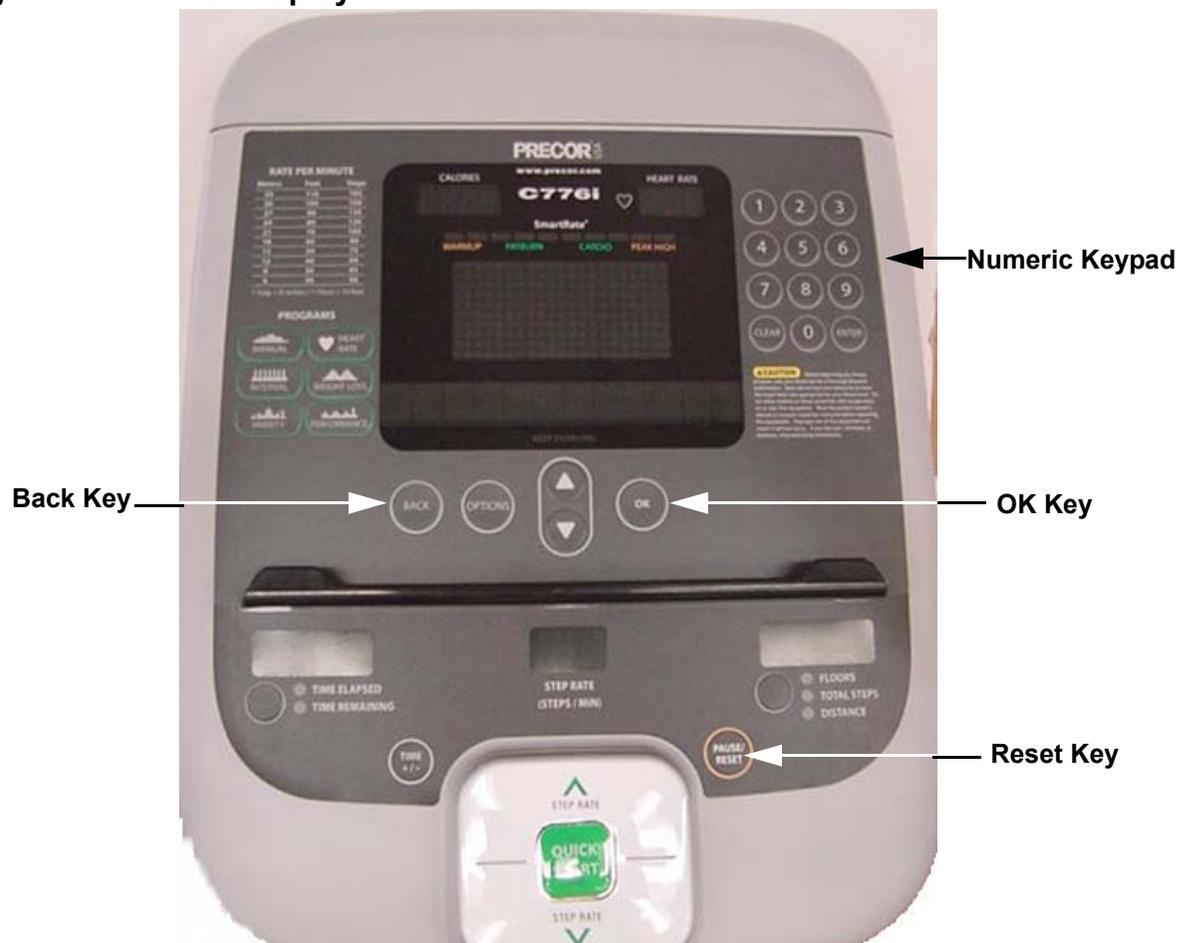
3. Press the **OK** key, the upper most group of LED's will illuminate on the display. Check the display to ensure that all LED segments are illuminated.
