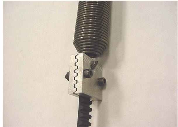
4. Remove the return spring from the other belt clamp. Remove the bolts that fasten the belt clamp to the belt and remove the belt from the clamp.
