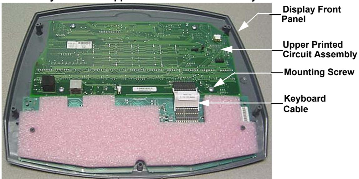
4. Remove the four screws that fasten the upper printed circuit assembly to the display front panel.
